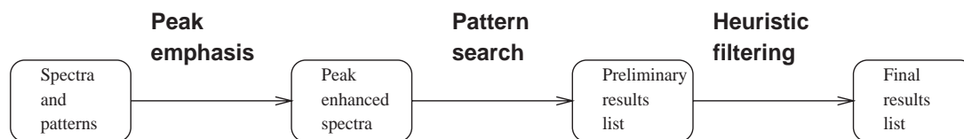
Fig. 2. Program flow diagram. The input required by the program consists of spectra and pattern files . Peak emphasis is a filtering operation which emphasises genuine peaks in selected portions of the spectra (regions of interest). Pattern search exhaustively explores the chemical shift space for peak patterns within the regions of interest (see also Fig. 4). A heuristic filter applies rules typically used by spectroscopists in order to penalise or remove unlikely results.
